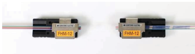
Figure 8. Ribbon Stripped and Cleaved
